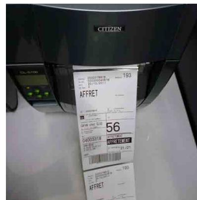
CL-S700 models are designed for ease of use - even in environments where space is limited. This avoids having to moving the printer to load media or switch access. The most common operations are accessible from the front of the printer. Paper or even tape can be loaded extremely fast.
